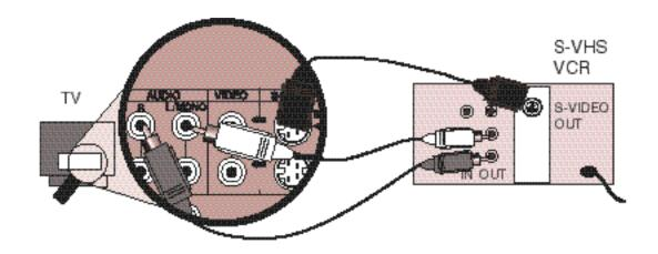
Keep the audio connections the same as for a non-S-VHS VCR or camcorder (page 9), and use the special S-VHS cable that came with the VCR or Camcorder. (This illustration is of an S-VHS VCR hookup — the same connections will apply for an S-VHS camcorder.)
